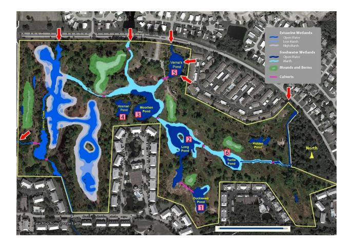
For the freshwater system, the work involved expanding several ponds, adding gradual sloping sides, and planting more than 60,000 wetland plants to help filter the water. With a few exceptions, for trail crossings and at the Duckweed Pond outflow, the underground culverts between the various ponds were removed and open flow ways were created.
