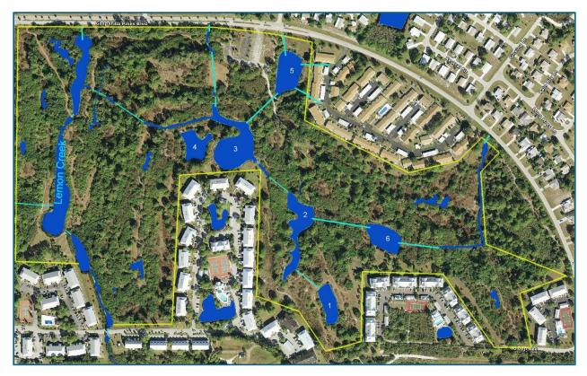
Starting on the east side, Pond 1 (Duckweed Pond) received treated sewage effluent through underground pipes from the Sandalhaven sewage treatment plant located to the south of the preserve. It was connected to Pond 2 (Long Pond) via an underground culvert (depicted in turquoise on the map).
